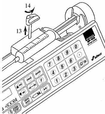
13. Lift the syringe clamp to its upper position.
