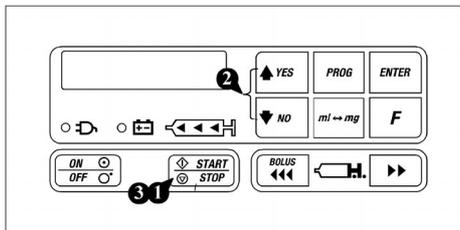
1. Press the START/STOP key. Segments of the indicator begin to flash sequentially.
