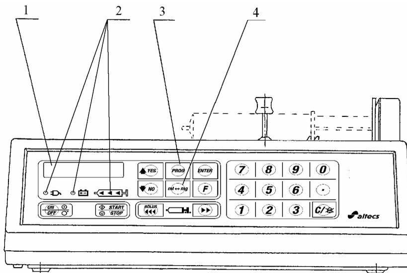
1. Display                      2. Indicators                      3. Keypad                      4. Key to select dimensions of parameters
