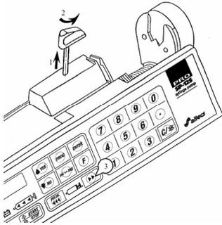
1. Lift the syringe clamp to its upper position.
