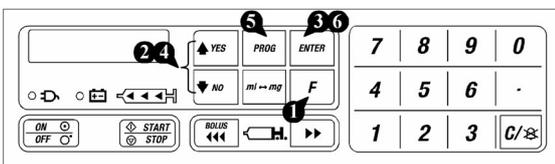
Programmed parameters may be modified only when the infusion is stopped (Infusion rate can be changed (Titration) during infusion as well as in the stop mode).
