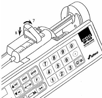
The syringe size sensor determines the syringe size automatically. The following message is displayed:
