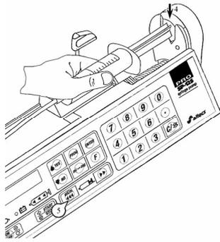
4. Insert the syringe push-button into the syringe driver arm slot to the depth to ensure minimal distance between the syringe barrel and the pump body.
