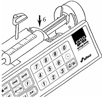
6. By pressing the syringe barrel and push-button down, insert fully the syringe finger grips and push-button into corresponding pump slots.
