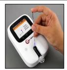
10. When the control activation solution is properly applied and detected, the flashing green light will turn off, and the meter will display 'Testing Please Wait'.
