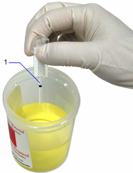
Figure 18 Filling the capillary with urine
